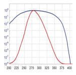
Determination of the absolute spectral responsivity of sglux sensors including calibration certificate according to DAkkS-DKD-MB3.
